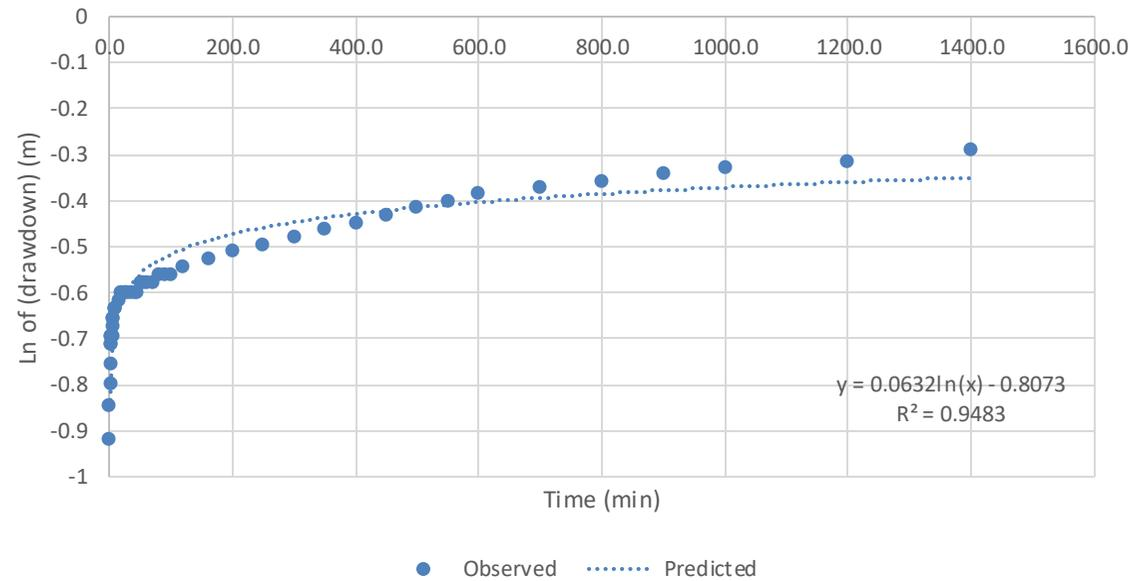
Figure 3.2 Graph log (drawdown) versus Time in minutes with predicted log regression line when Q=51.6m<sup>3</sup>/hr.
