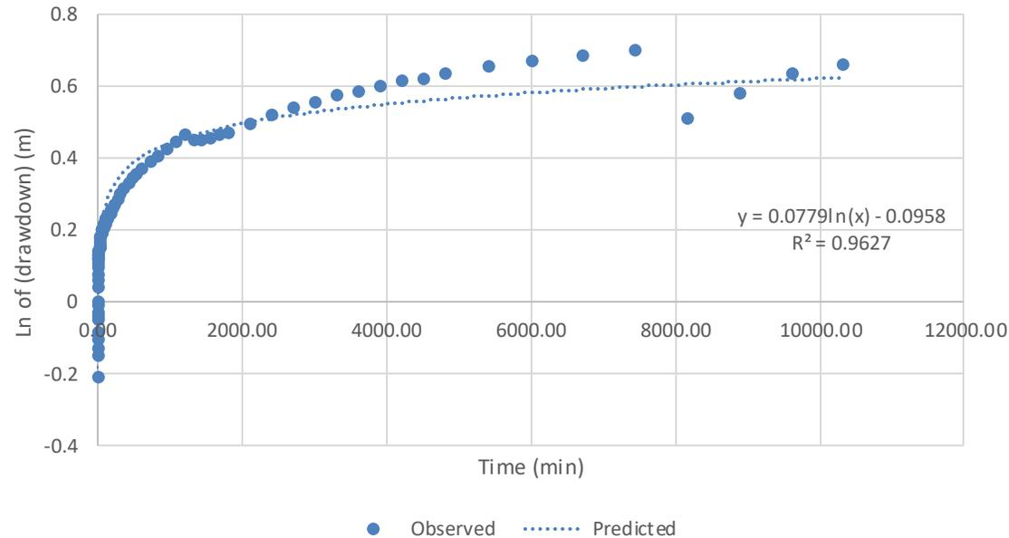
Figure 3.3 Graph log (drawdown) versus Time in minutes with predicted log regression line when Q=90.2m<sup>3</sup>/hr.
